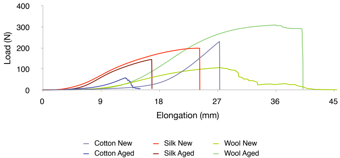
Figure 6.10: New and aged fabrics load/elongation curves
