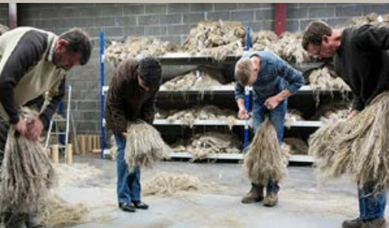
Fig. 9. Scutching linen fibers (also known as heckling) prior to spinning. Today, companies like Leitner Leinen in Austria can use machinery to assist in zero-waste linen production.
