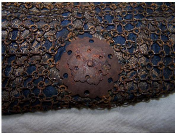
Fig. 8. This detail of mail on a *kote* clearly shows that the metal has started to rust. Fortunately it is not yet causing damage to the silk textile below. If this artifact is exposed to high RH and temperature fluctuations, the rust will worsen and begin to affect the neighboring materials.
