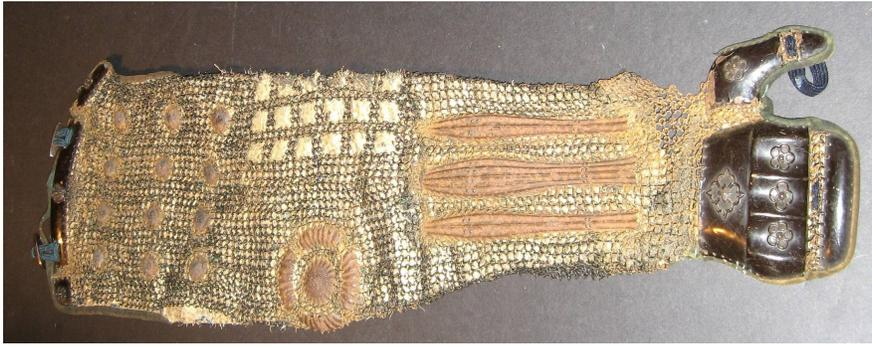
Fig. 3. The silk and hemp textiles on this *kote* are in good condition. The mail has rusted but the more heavily lacquered metal on the hand has not.
